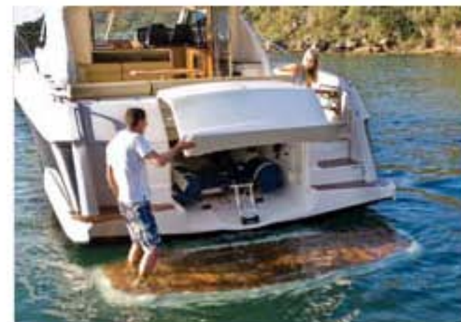
ABOVE: The tender garage was a must-keep feature from the 4700, plus the designers have made room for a 3.1-metre Zodiack between the Zeus legs.
